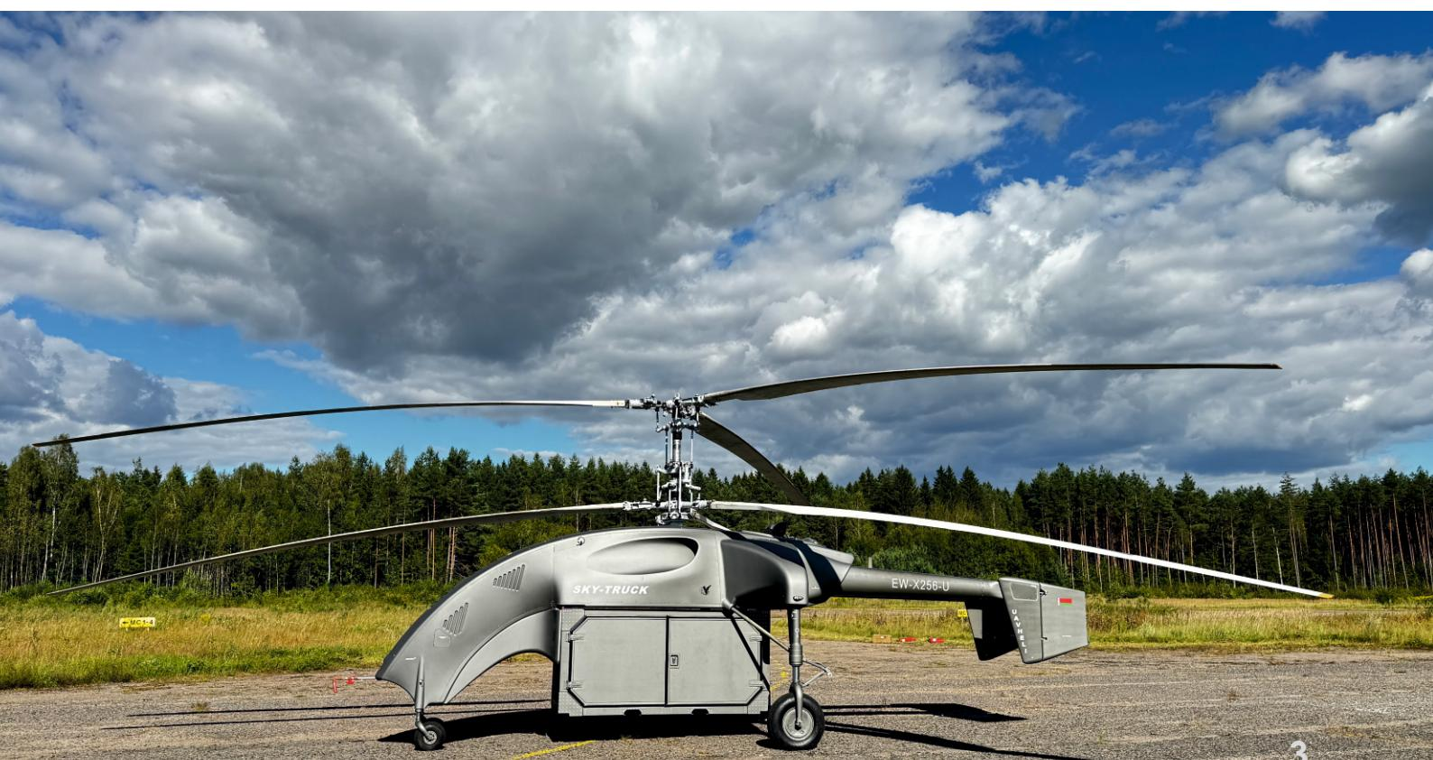
The UAV is equipped with an avionics complex that provides in automatic mode: takeoff, flight, landing of the UAV with the possibility of hovering over the object to complete the mission, as well as control of the payload and the onboard part of the data transmission system.
