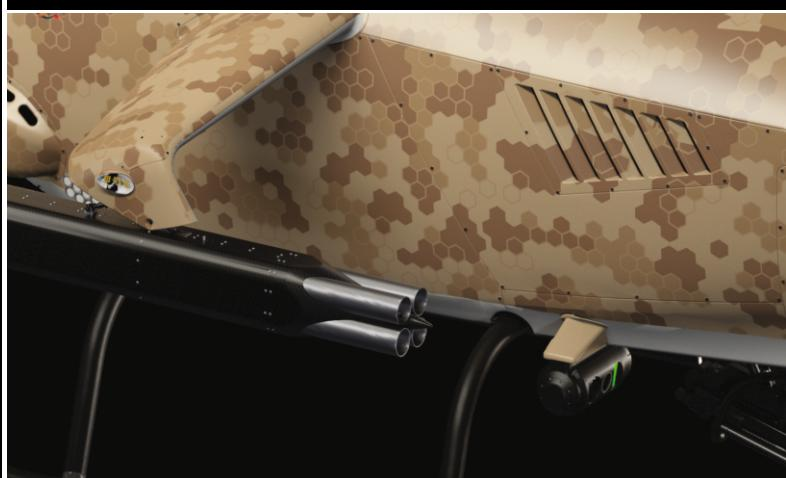
Two UB-4 units for four S-5 missiles each are mounted on two automatically adjustable beam holders of auxiliary wings.
