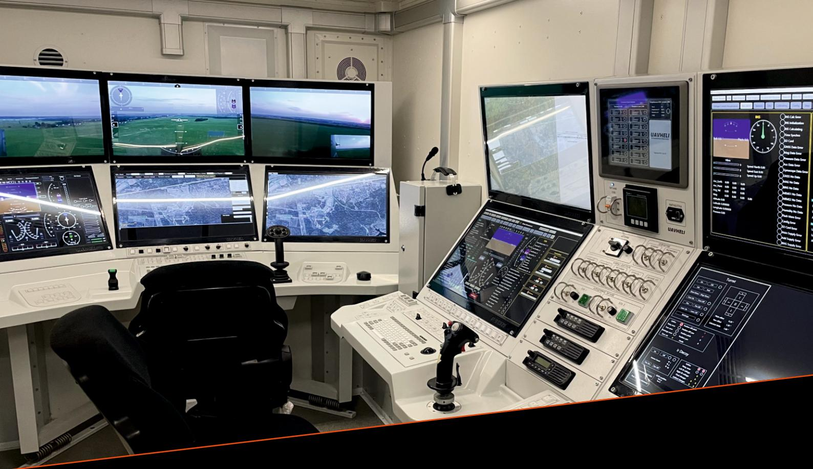
The ground control station has four automated workstations for two UAV operators and two payload operators.
