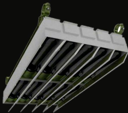
Under the fuselage, it is possible to install a bomb cassette BK-2.5-16 designed for round-the-clock use of 16 anti-tank aerial bombs using the geographic coordinates and an optoelectronic aiming system.
