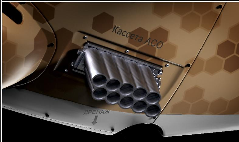
Combined ejection devices are installed, which are designed to interfere with heat-seeking missiles.
