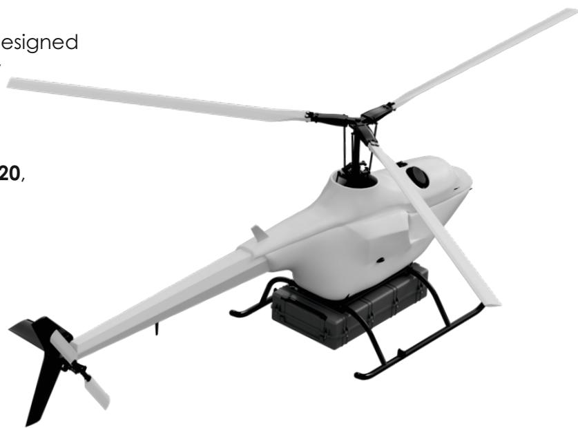
The **FALCON** unmanned helicopter is an optimal solution of the task of delivery of goods weighing up to 200 kg to hard-to-reach places.
