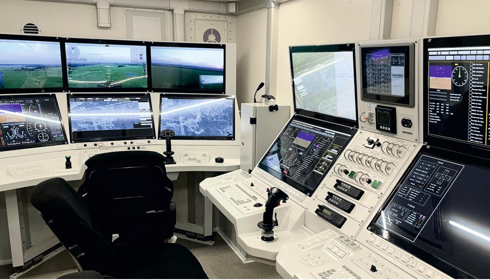
The Ground control station has four automated workstations for two UAV operators and two technicians.
