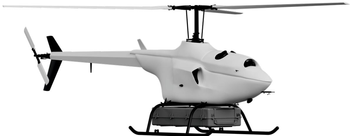
The helicopter is equipped with an avionics complex that provides automatic take-off, flight and landing of an unmanned aerial vehicle with the ability to hover over the mission site.
